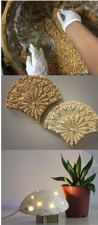
Figure 1. Our mycelium biofabrication methods and artifacts, from top to bottom: (A) hand-sculpting mycelium forms (B) Replicas of 3D prints grown out of mycelium (C) 'Fibrous Lights' with micro LEDs embedded during the growth process.
