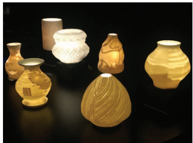
Fig. 1. PLA plastic, 3D-printed lithophanes created with Lithobox. Custom images were mapped and extruded along the lithophanes' inner and outer surfaces and can be seen when lit from within. Photo taken at the 2019 Arts Track Exhibit of the ACM International Conference on Tangible, Embedded and Embodied Interaction (TEI). (© Jennifer Weiler)
