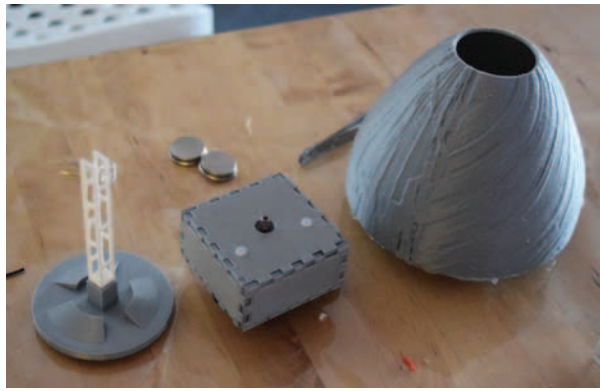
Fig. 5. Example of a lithophane with 3D-printed assembly parts: base and support tower, MakerCase box containing Arduino rotator and 3D-printed lithophane. The total height of the assembled lithophane and support structure is 7.5 in, composed of PLA plastic. (© Jennifer Weiler)
